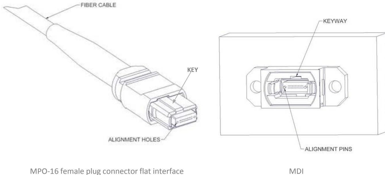
Figure xx-c – MPO-16 female plug connector flat interface and MDI
