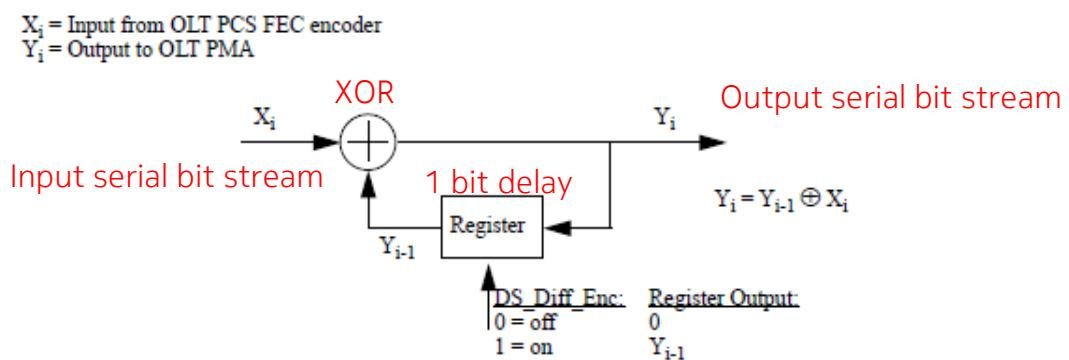
Figure 142-19—Differential encoding
