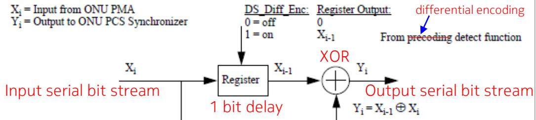
Figure 142-20—Differential decoding
