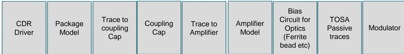
For 56Gbaud, every detail needs to be modeled. Every time there is a mode conversion, there is possibility of pre-cursor distortion. As the signal propagates, there are multiple points where the mode conversion could be happening and thus leading to variation in pre-cursor. Also the traveling amplifier and modulators will have varying pre-cursor due to various laws of physics they are build on.
