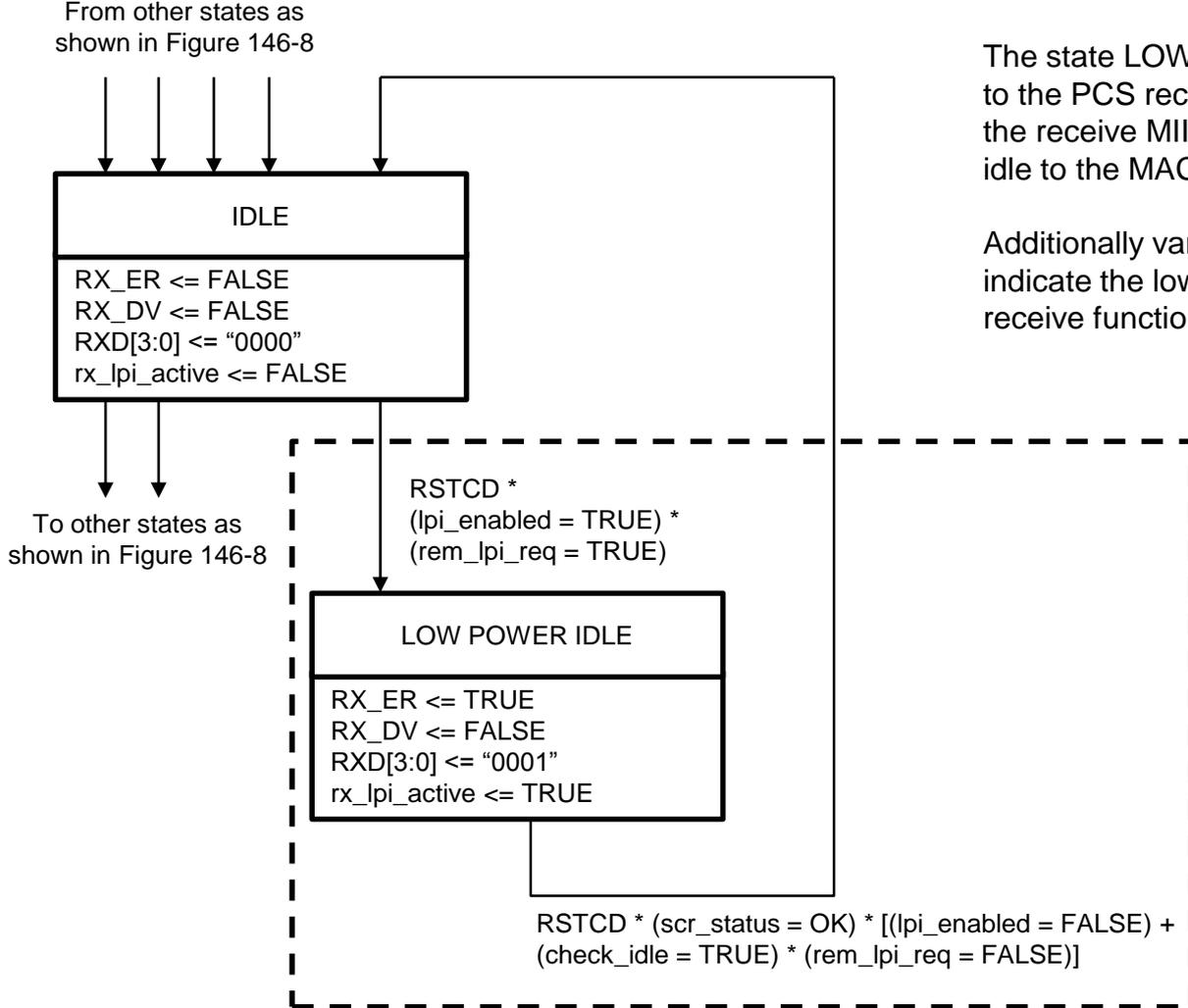
The state LOW POWER IDLE needs to be added to the PCS receive state diagram. In this state the receive MII signals are set to signal low power idle to the MAC.
