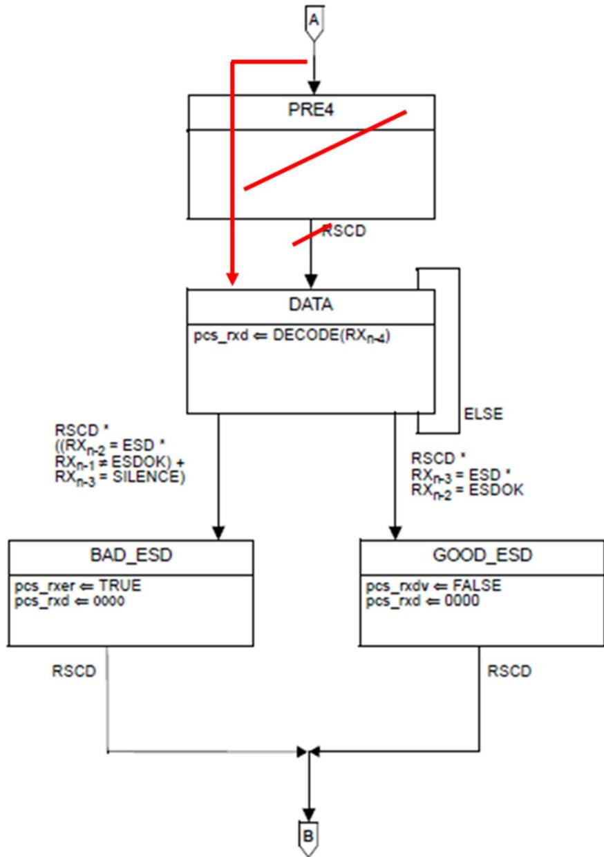
Figure 147-7—PCS Receive state diagram (2 of 2)
