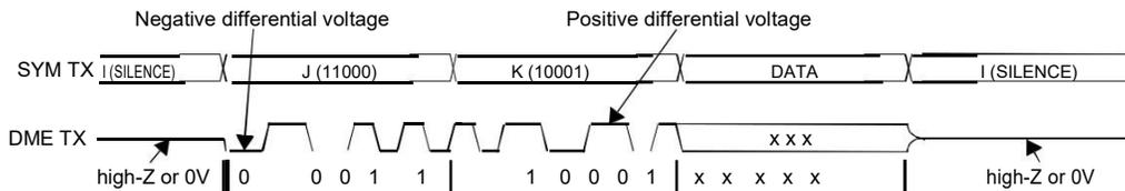
Figure 147-9—Example DME encoding of 5B symbols
