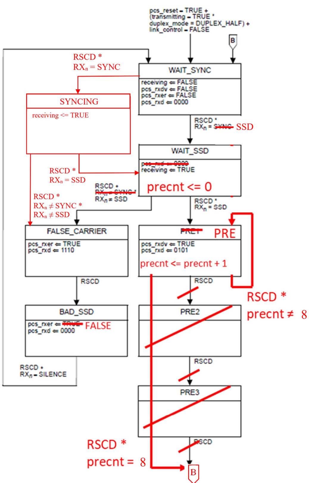
Figure 147-6—PCS Receive state diagram (1 of 2)
