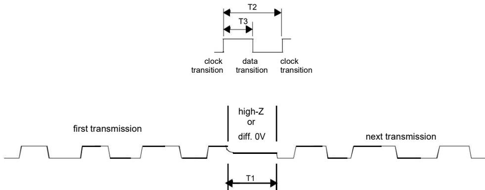
**Figure 147-8—DME Encoding Scheme**
