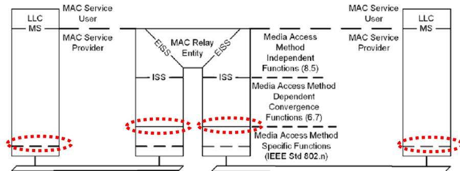
NOTE—The notation "IEEE Std 802.n" in this figure indicates that the specifications for these functions can be found in the relevant standard for the media access method concerned; for example, n would be 3 (IEEE Std 802.3) in the case of Ethernet.
