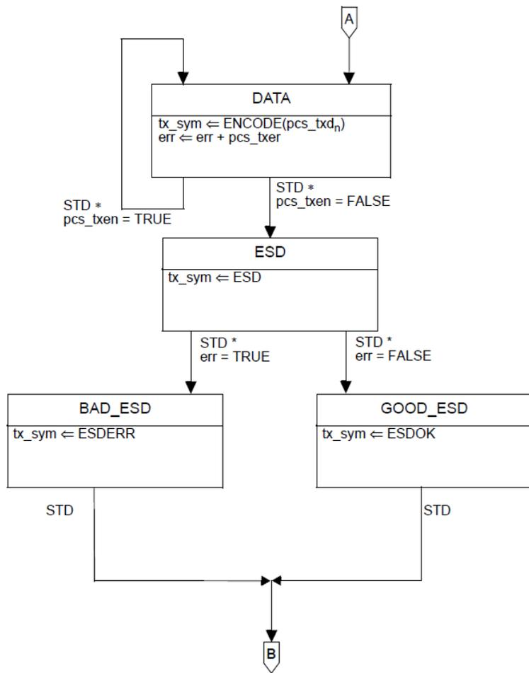
Figure 147-5—PCS Transmit state diagram (2 of 2)
