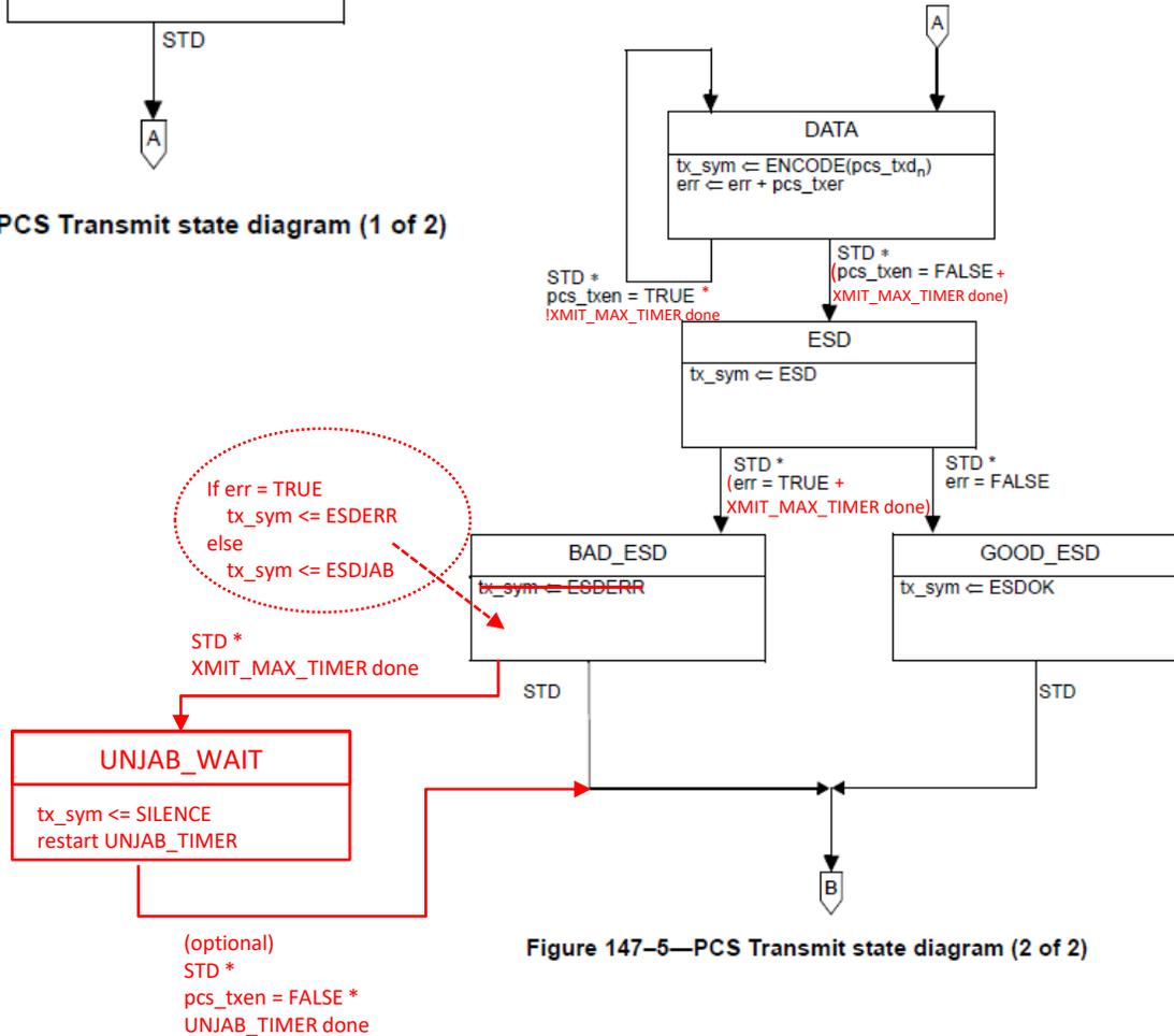
Figure 147-5—PCS Transmit state diagram (2 of 2)
