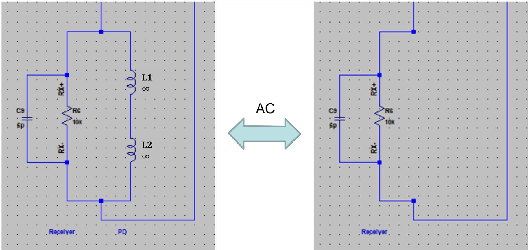
Not including inductors is the same as having an infinite inductance at AC frequencies
