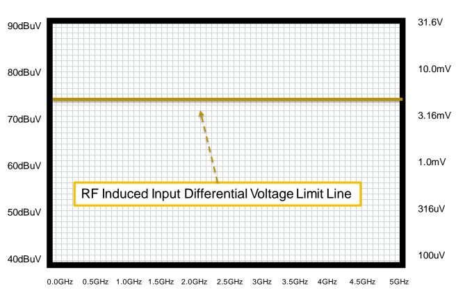
The limit line used for the differential voltage magnitude at the PHY input induced by the RF fields coupled to the STP cable, which was used for the analysis
