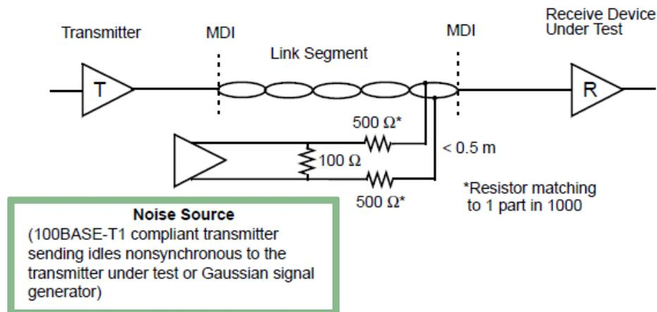
Figure 96-26—Alien crosstalk noise rejection test setup
