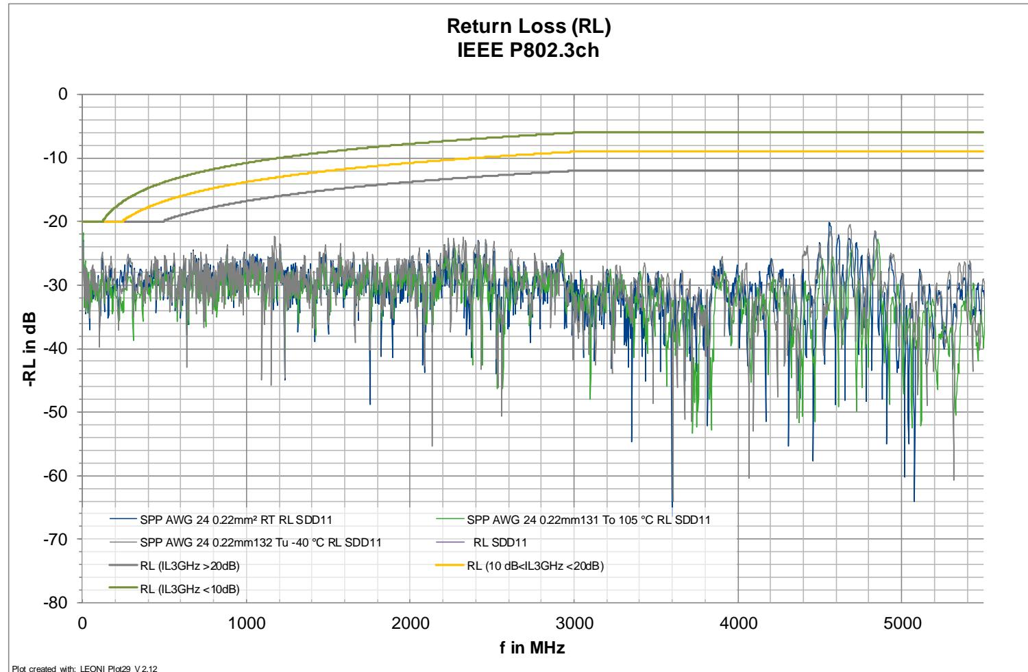
No significant change in Return loss due to temperature change.
