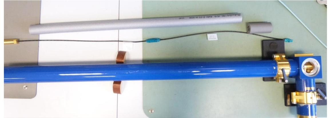
Coupling- and screening attenuation reference cable assembly
