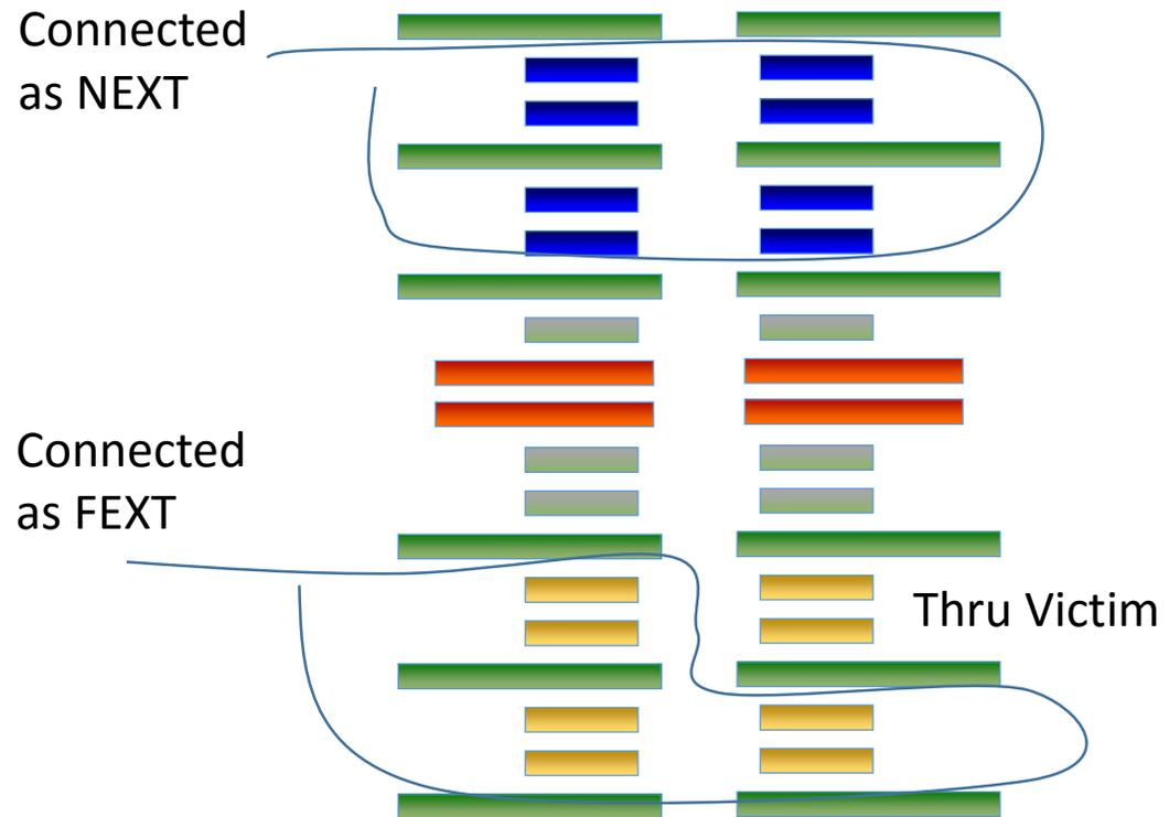
Tx and Rx on separate cable bundles makes for very low NEXT
