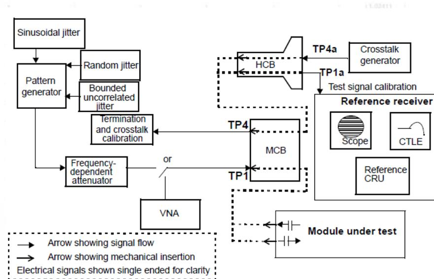
Figure 120E-12—Example module stressed input test
