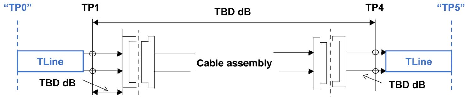
COM for the calculated TP0 to TP5 channel must be no less than  $COM_{min}$ . This implies backplane and cable assembly TP0 to TP5 channels are inter-changeable.
