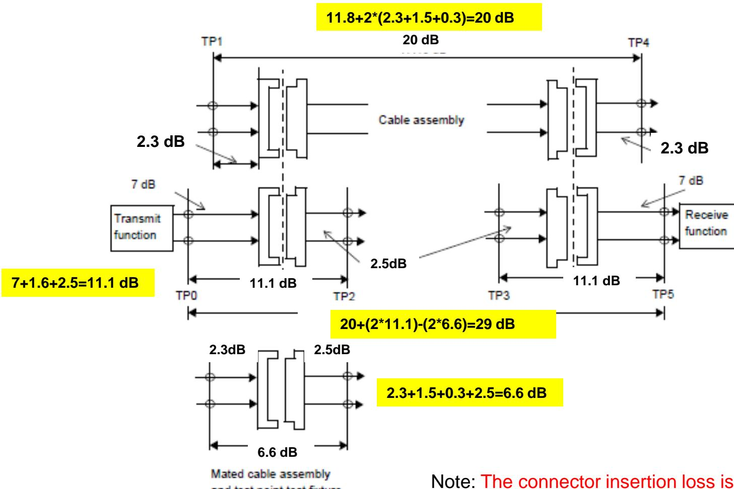
Note: The connector insertion loss is 1.5 and via allowance of 0.3 dB for the mated test fixture. The host connector is allocated 0.1 dB for implementation allowance.
