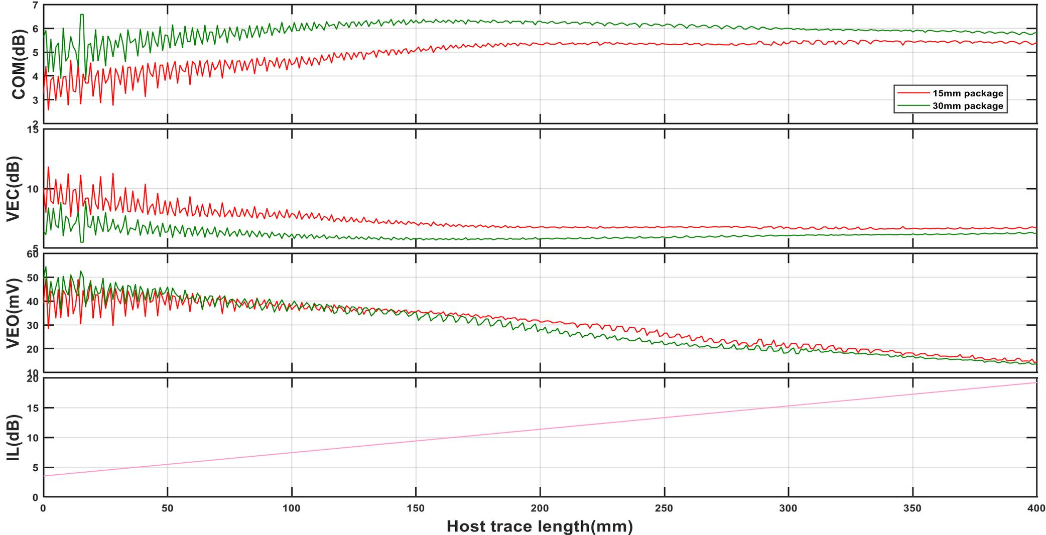
Longer package trace (more loss) is better for COM and VEC although slightly worse for VEO
