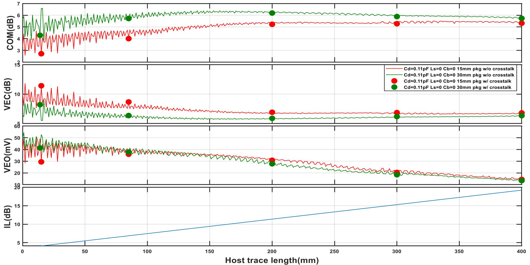
Crosstalk is not a significant degradation for this connector with these trace lengths.
