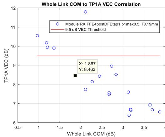
TX FIR is set by RX C. TP1a VEC threshold is 9.5 dB
