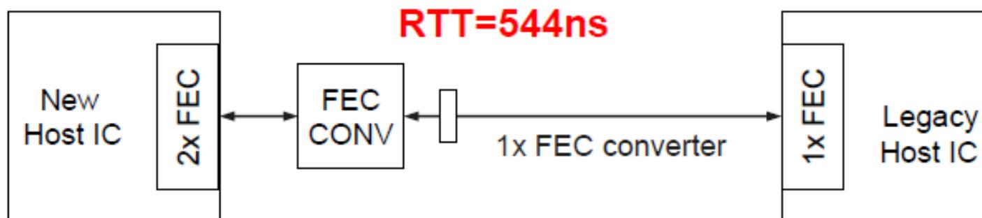
\*RTT=2x 50G decoding latency + 2x 100G decoding latency + 20ns wire latency.
