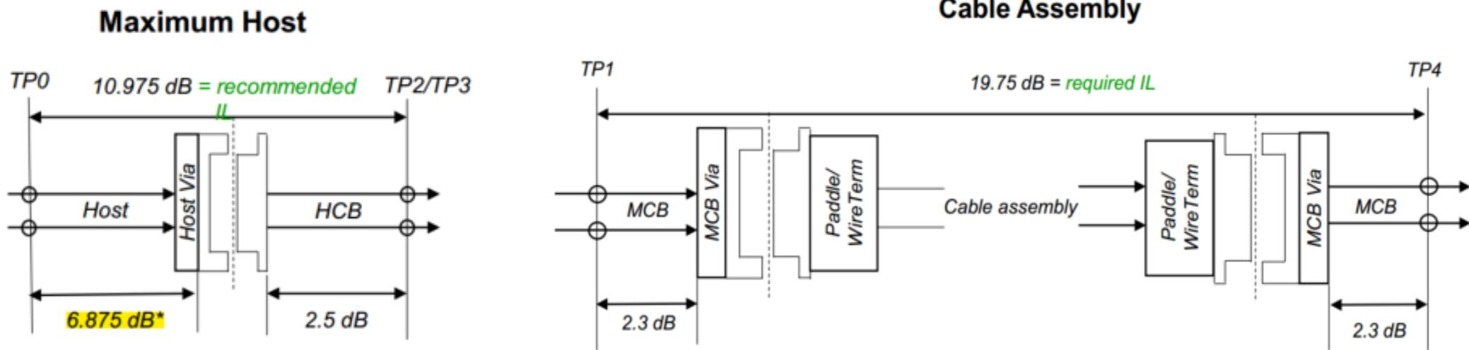
Note: The 6.875 dB includes via allowances for BGA and connector footprint
