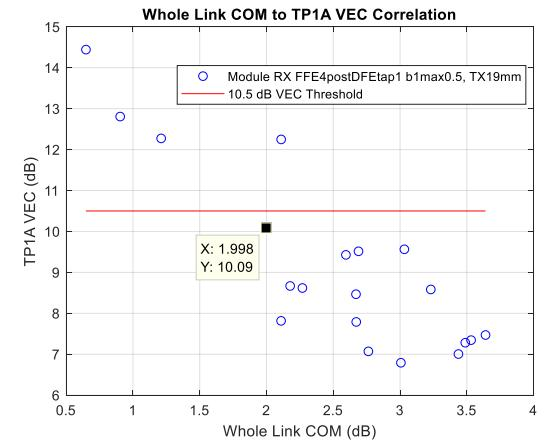
TX FIR is set by RX D2. TP1a VEC threshold is 10.5 dB
