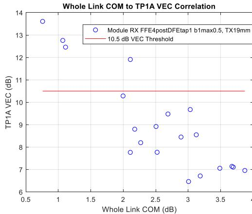
TX FIR is set by RX C2. TP1a VEC threshold is 10.5 dB
