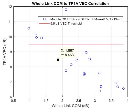
TX FIR is set by RX C. TP1a VEC threshold is 9.5 dB
