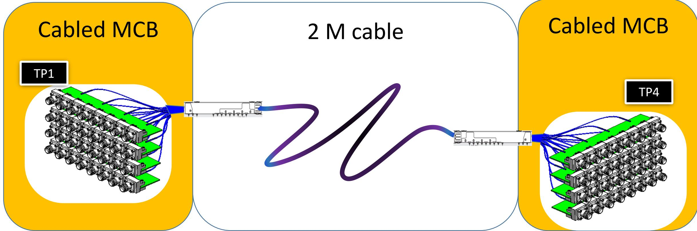
Cable assembly model is 19.75 dB IL at 26.56 GHz
