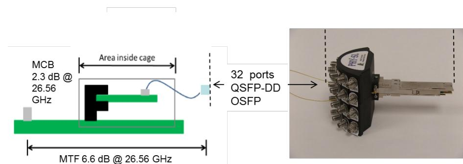
Note: 2.3 dB MCB PCB includes test point IL
