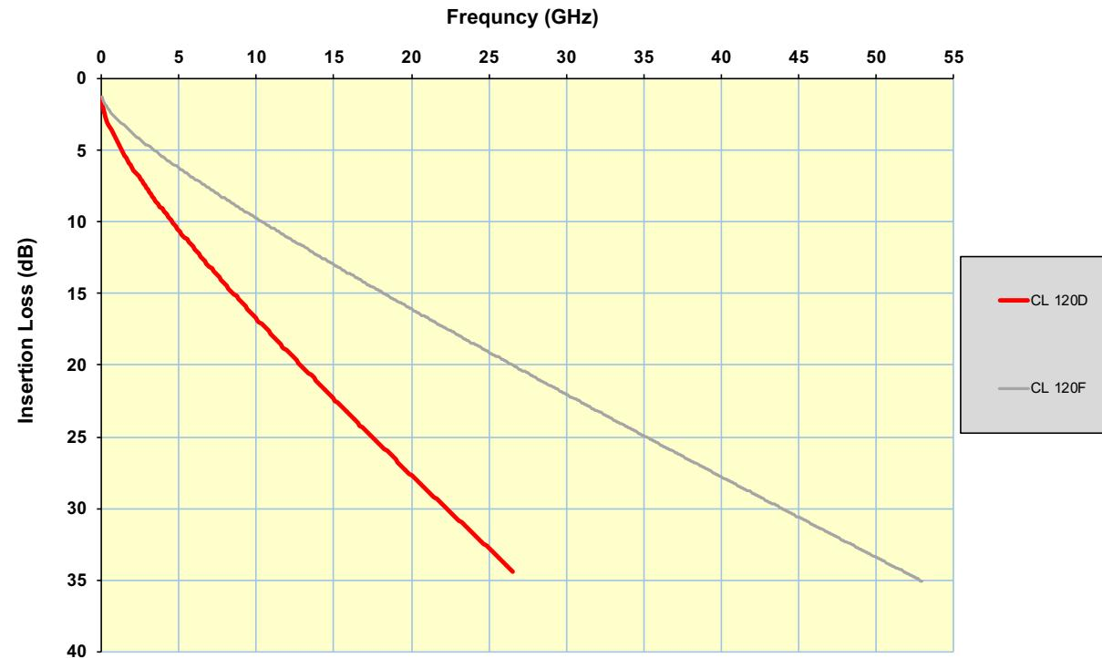
$$\text{Insertion\_Loss}(f) = 1.083 + 1.25\sqrt{f} + 0.47f \quad 0.01 \leq f \leq 50 \text{ GHz}$$
