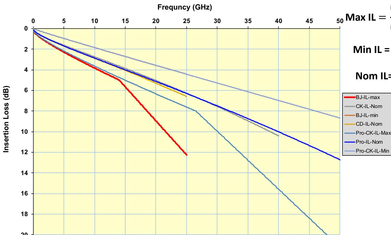
$$\text{Max IL} = \begin{cases} (0.12 + 0.475\sqrt{f} + 0.221f) \times 0.9503 \text{ dB } 0.01 \leq f \leq 26.55 \text{ GHz} \\ 6.9505 + 0.562f \quad 26.55 < f \leq 50 \text{ GHz} \end{cases}$$
