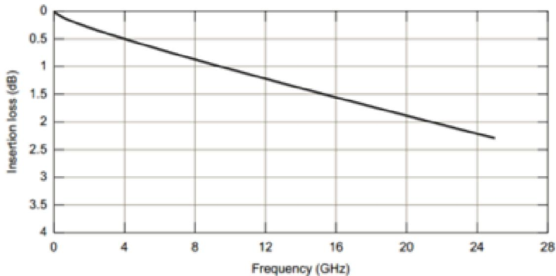
Figure 93-3—Test fixture reference insertion loss
