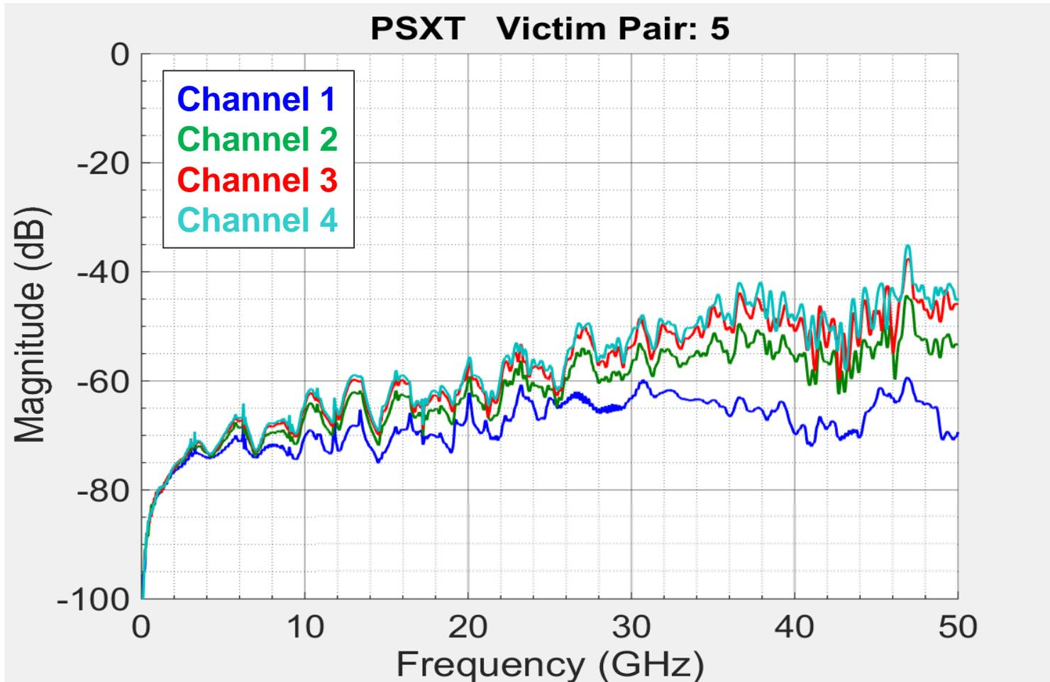
NOTE: Crosstalk performance is expected to degrade with the inclusion of a multi-pair BGA via model
