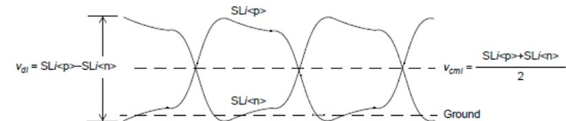
Figure 93-6—Transmitter output voltage definitions
