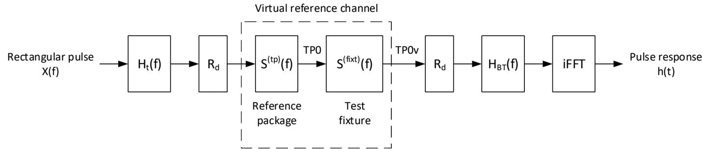
Note: the transmitter reference package uses the maximum trace length specified in the referring clause.
