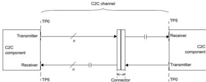
Note—The number of lanes  $n$  is equal to 1 for 100GAUI-1, 2 for 200GAUI-2, and 4 for 400GAUI-4.
