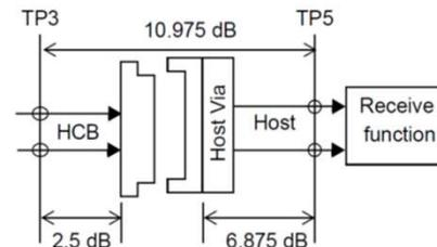
NOTE—The 6.875 dB IL includes allowance for BGA and connector footprint vias.
