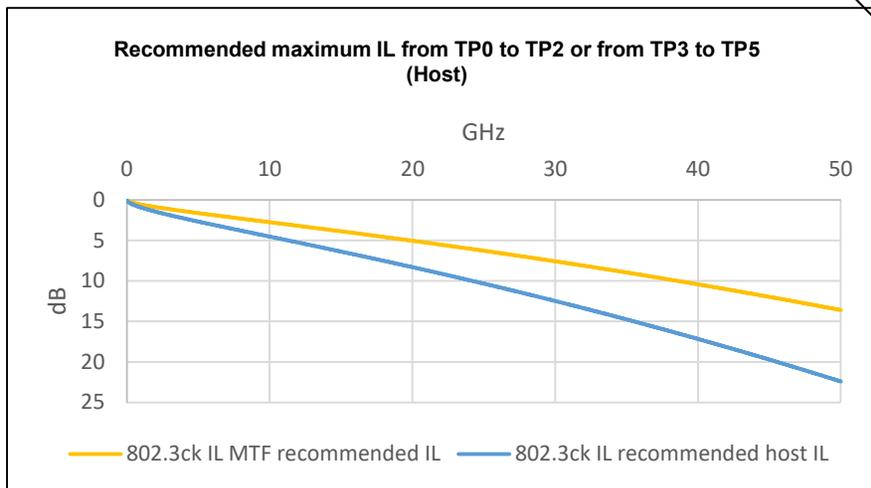
$$IL_{MTF}(f_{GHz}) = 0.9502 * (0.471 * \text{SQRT}(f_{GHz}) + 0.1194 * f_{GHz} + 0.002 * (f_{GHz}^2))$$
