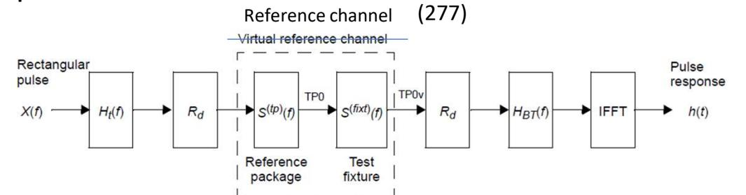
NOTE—The transmitter reference package uses the maximum length specified by the referring subclause.
