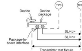
Figure 94-10—Transmitter test fixture and test points
