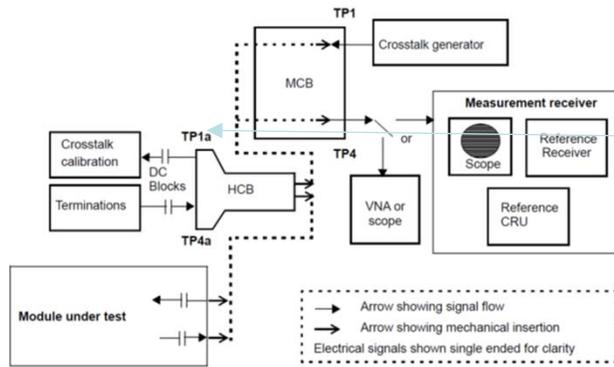
Figure 120G-7—Example module output test configuration
