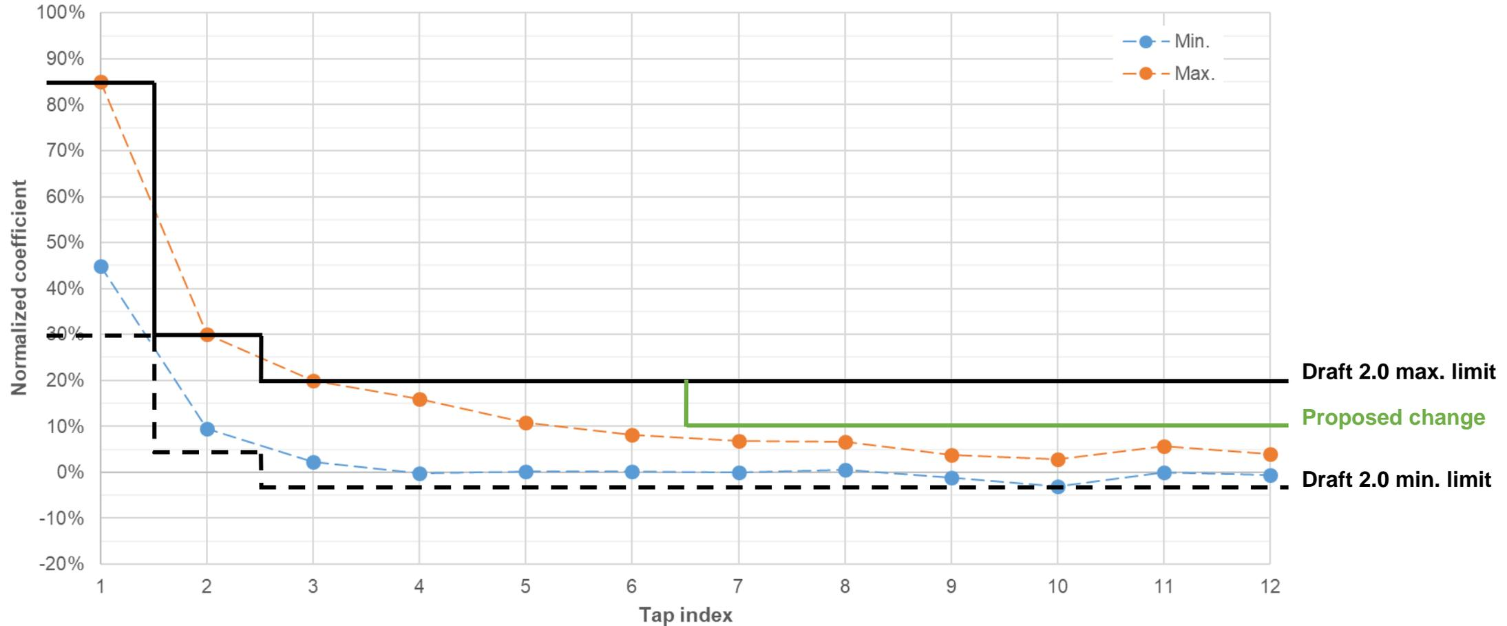
101 channels with COM  $\geq$  2.5 dB, 2 tests (package transmission line length) per channel, 202 coefficient sets
