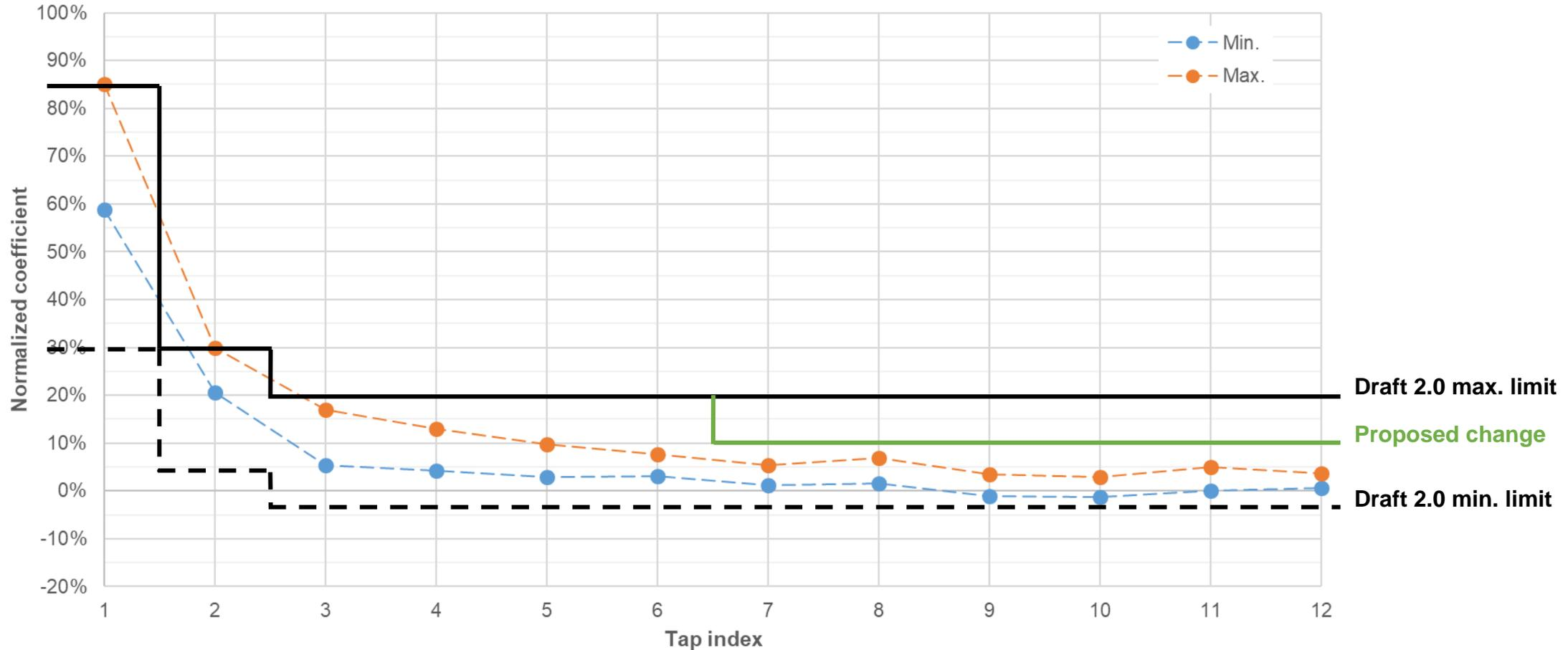
17 channels with  $\text{COM} \geq 2.5$  dB, 2 tests (package transmission line length) per channel, specified host trace model added, 34 coefficient sets
