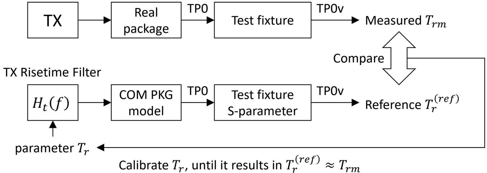
Figure 163-W – Calibration of risetime  $T_r$  at signal source against measured transition time  $T_{rm}$
