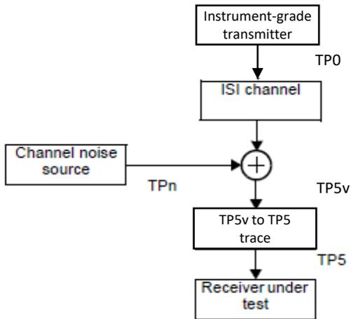
Figure 163-X – Interference tolerance test setup using an instrument-grade transmitter
