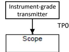
Figure 163-Y – Interference tolerance transmitter test setup for an instrument-grade transmitter
