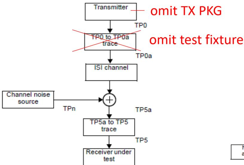
Figure 93C-2—Interference tolerance test setup
