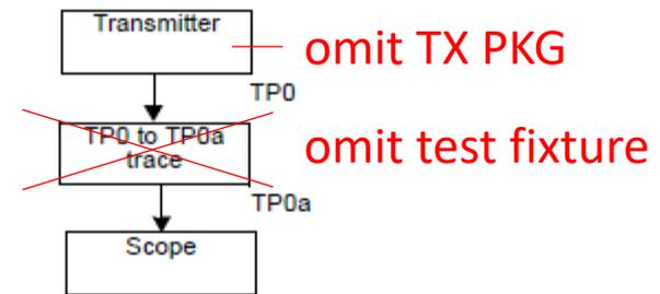
Figure 93C-3—Interference tolerance transmitter test setup
