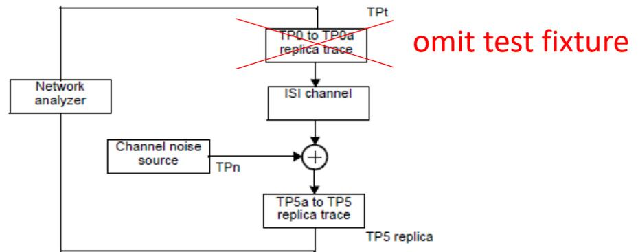
Figure 93C-4—Interference tolerance channel s-parameter test setup
