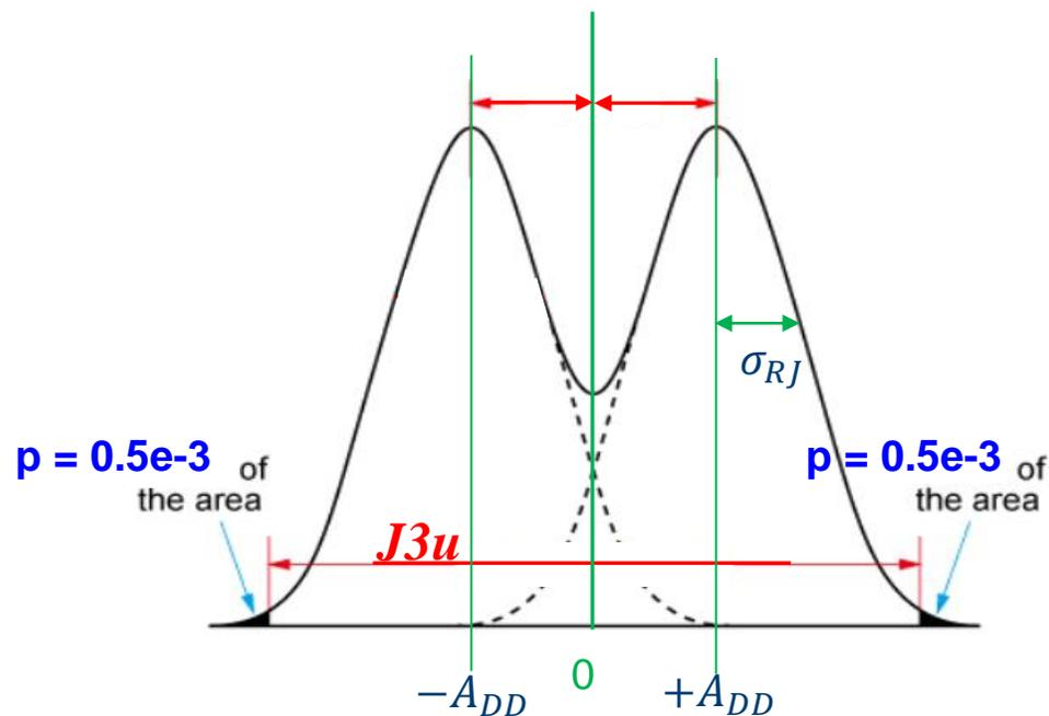
$$A_{DD} = \frac{\frac{J_{3u}}{2} + Q3 \sqrt{(Q3^2 + 1)J_{RMS}^2 - \left(\frac{J_{3u}}{2}\right)^2}}{Q3^2 + 1} \quad (802.3: 163-2)$$
