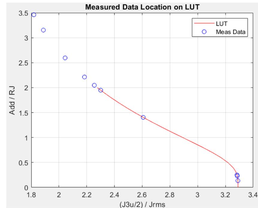
$(A_{DD}, \sigma_{RJ})$  estimation accuracy degrades when LUT does not cover
