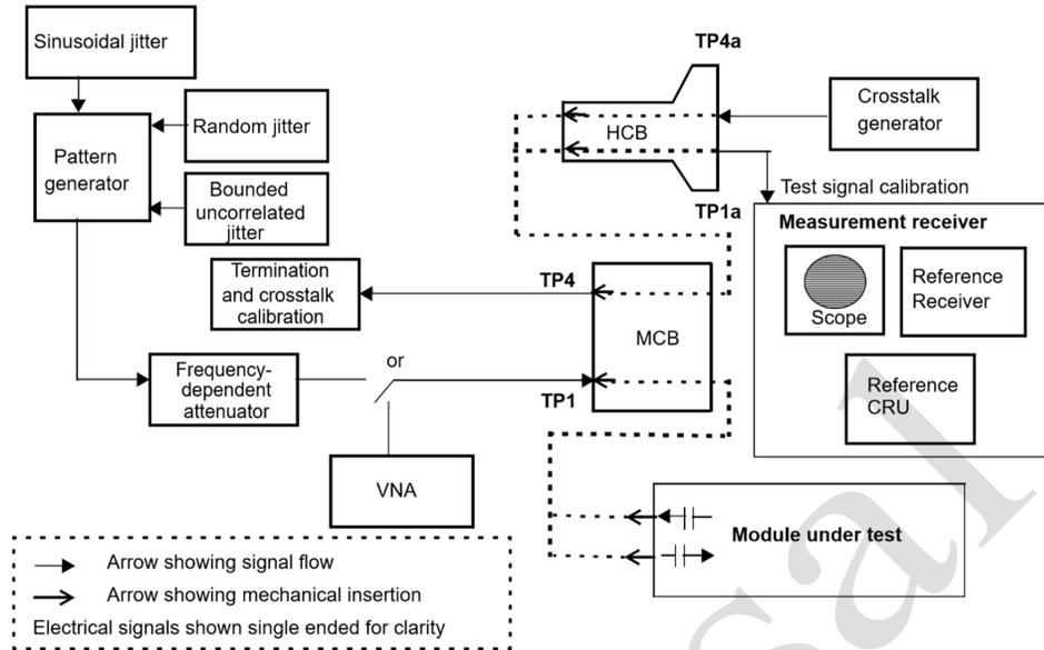
Figure 120G-10—Example module stressed input test setup
