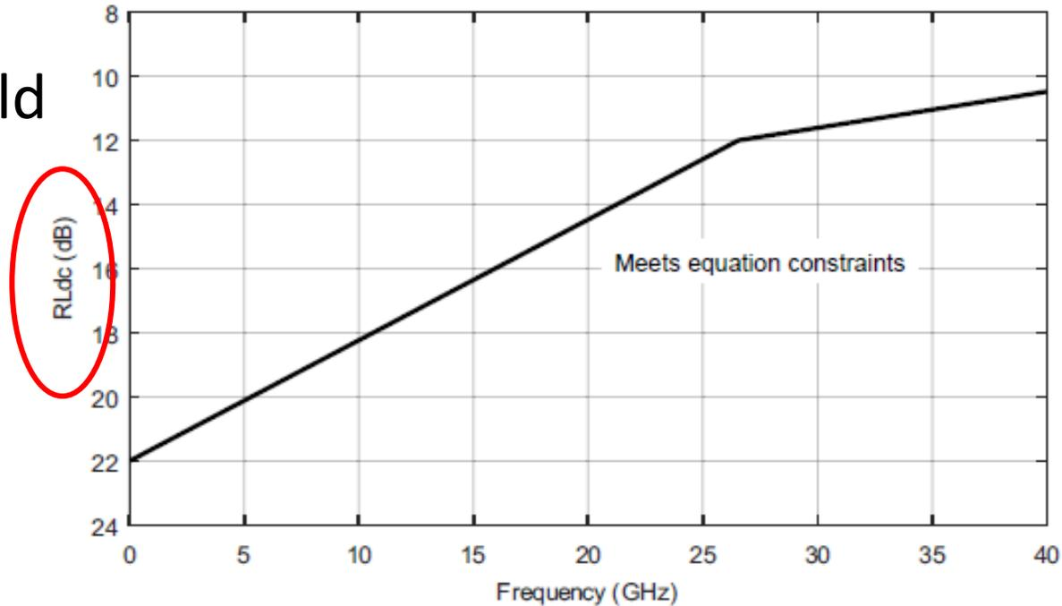
Figure 162-8—Cable assembly differential-mode to common-mode return loss
