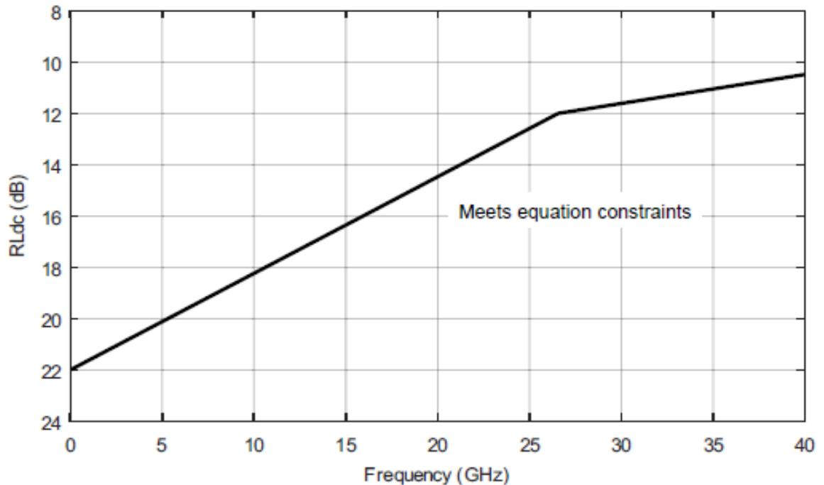
Figure 162-4—Transmitter common-mode to differential-mode return loss
