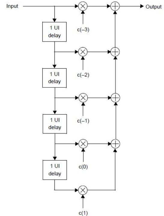
Figure 120F–3—Transmitter equalizer functional model
