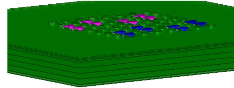
A simple estimated model for the via field underneath the silicon end-agent was created.
