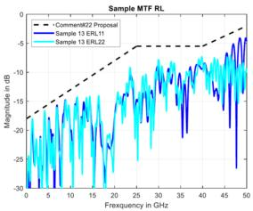
The difference caused by the limit line violation >45GHz is ~0.2dB ERL
