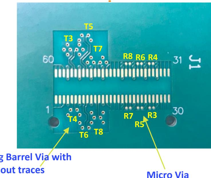
Long Barrel Via with Fan out traces
