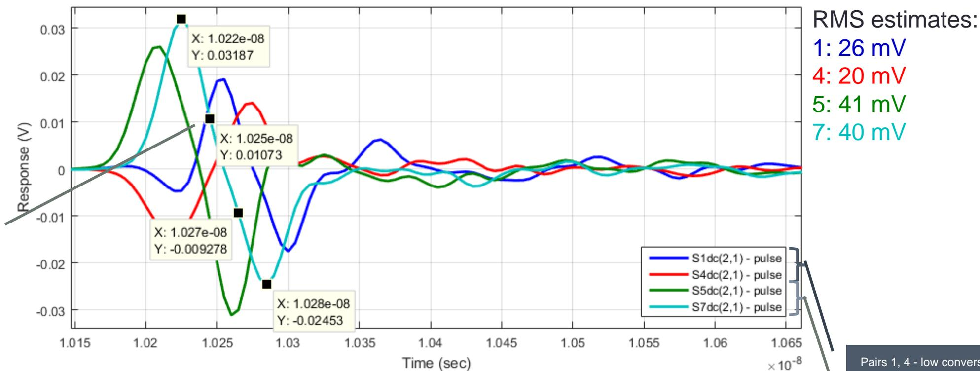
CM RMS estimated by taking the RSS of the positive and negative peaks of each pulse. Best case is 25 dB below the signal. Worst case is 18.7 dB below signal.
