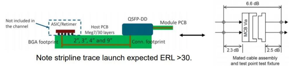
Chip to module block diagram for TP1a performance
