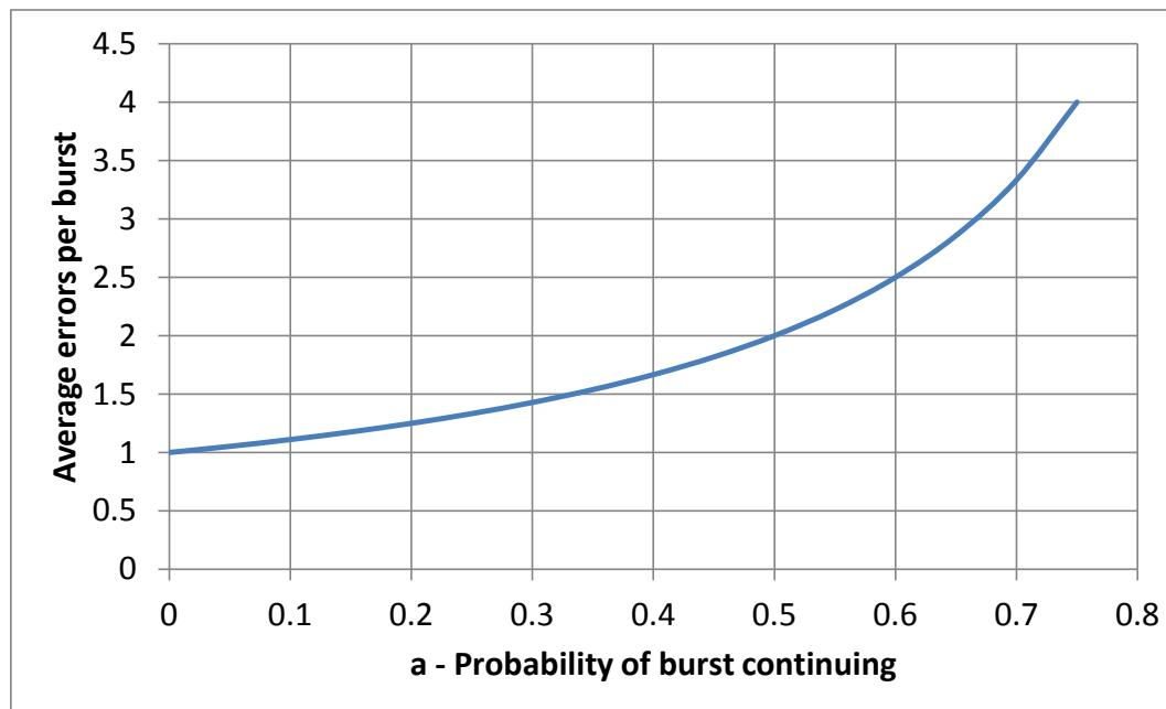
For  $a = 0.75$ , the  $BER_{in}$  including bursts is  $4 \times$  the  $BER_{in}$  due to noise.
