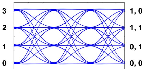
Since two of the eight possibilities result in both bits being correct, these states terminate the burst. Therefore for Gray coded PAM4, if a **symbol** is in error, the worst case probability that the next **symbol** is also in error is 0.75.
