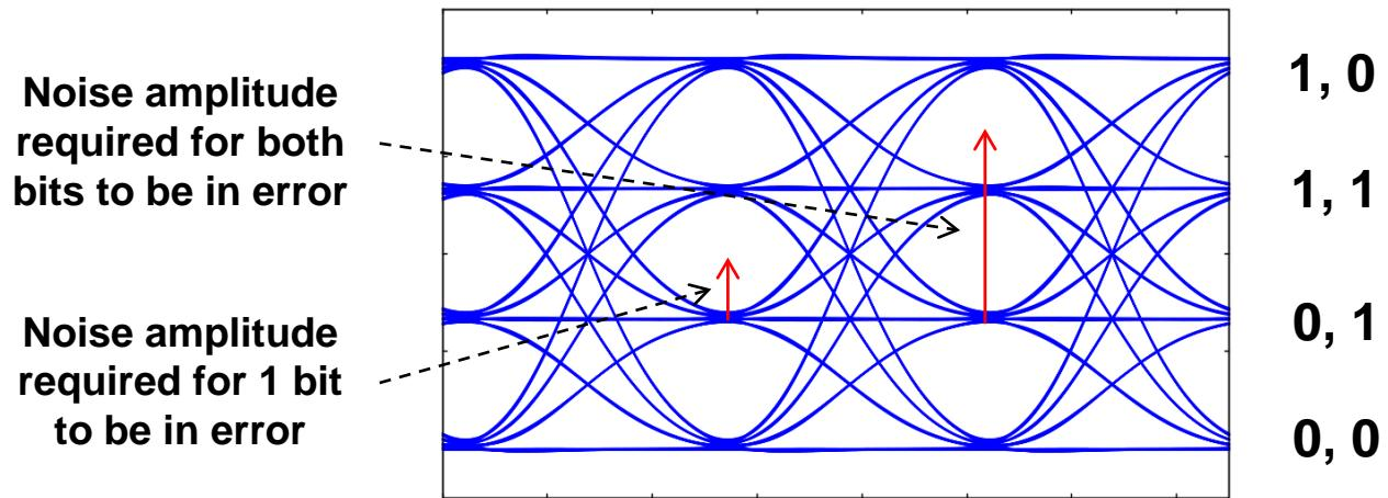
If noise causes any of the 4 levels to be mistaken for an adjacent level, this causes one of the two bits to be in error.
