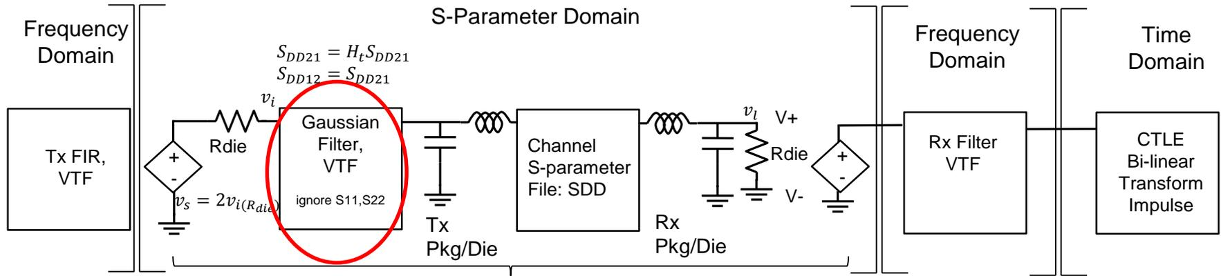
Cascade S-parameters and convert to VTF (XSR Die Model)
