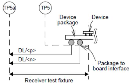
Figure 163–5—Receiver test fixture and test points
