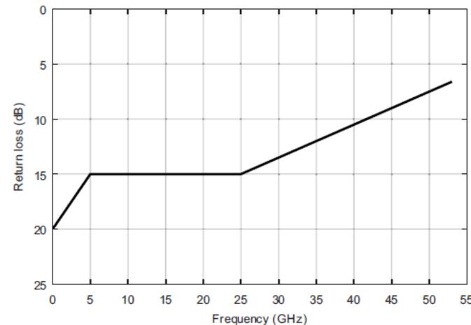
Figure 163-5—Test fixture reference return loss limit
