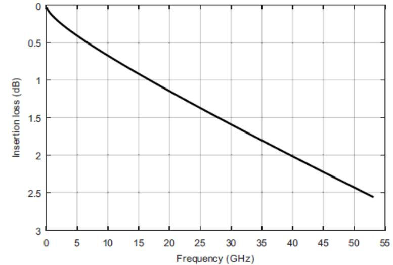
Figure 163-4—Test fixture reference insertion loss
