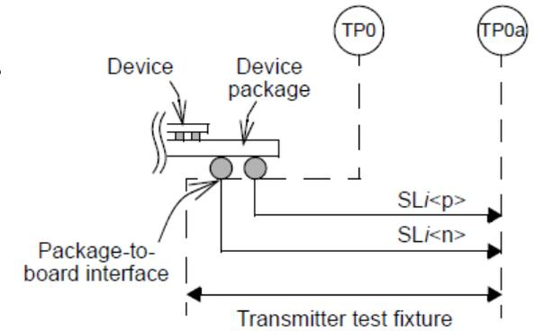
Figure 163-3—Transmitter test fixture and test points
