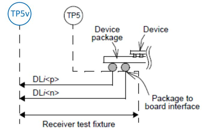
Figure 163–5—Receiver test fixture and test points
