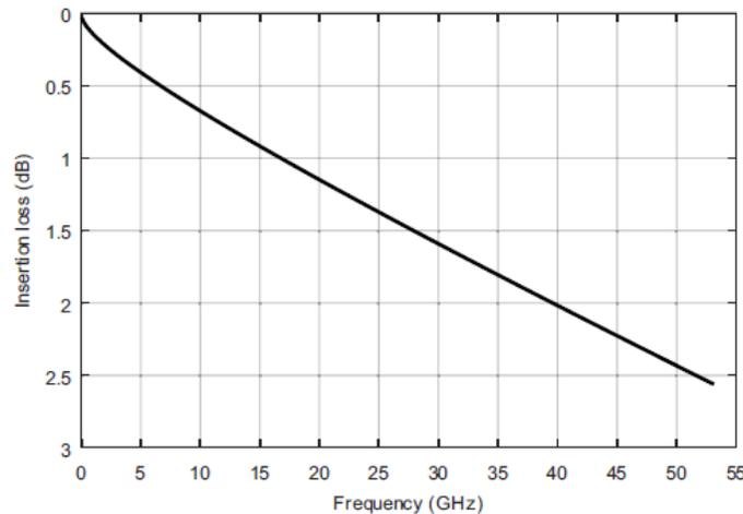
Figure 163-4—Test fixture reference insertion loss
