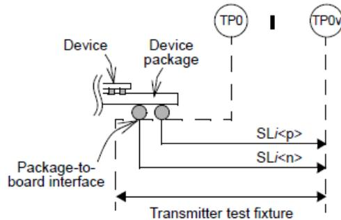
Figure 163–3—Transmitter test fixture and test points
