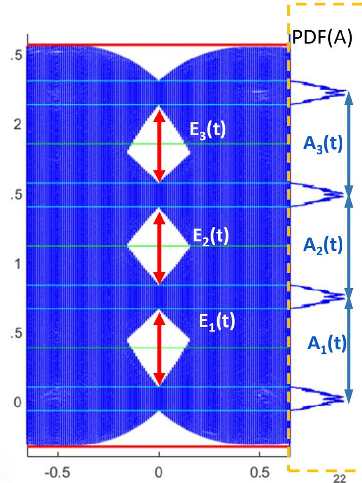
For non equalized channels previous equations can be simplified as shown in Journal of Lightwave Tech. Vol 34 (16) , April 2016
