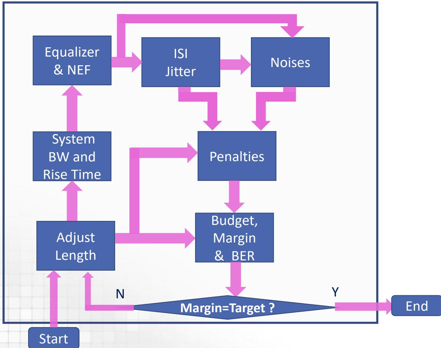
Adjust link length until margin equals zero (or a targeted value)
