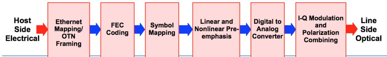
[Figure 11 - Transmitter Functional Diagram](#)
