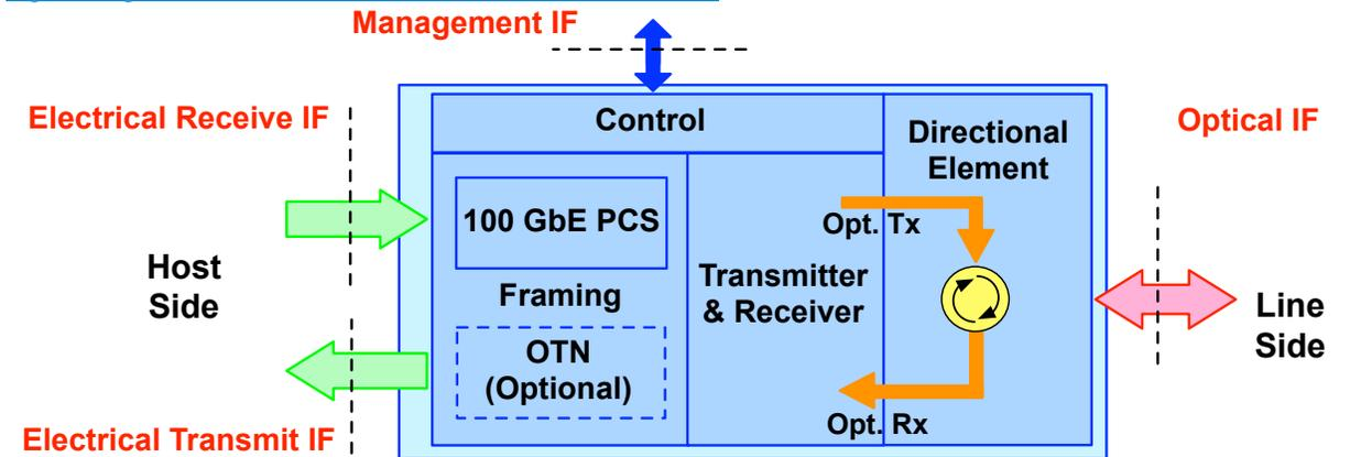
Figure 11– Single Optical Interface Transceiver Optical, Electrical and Management Interfaces
