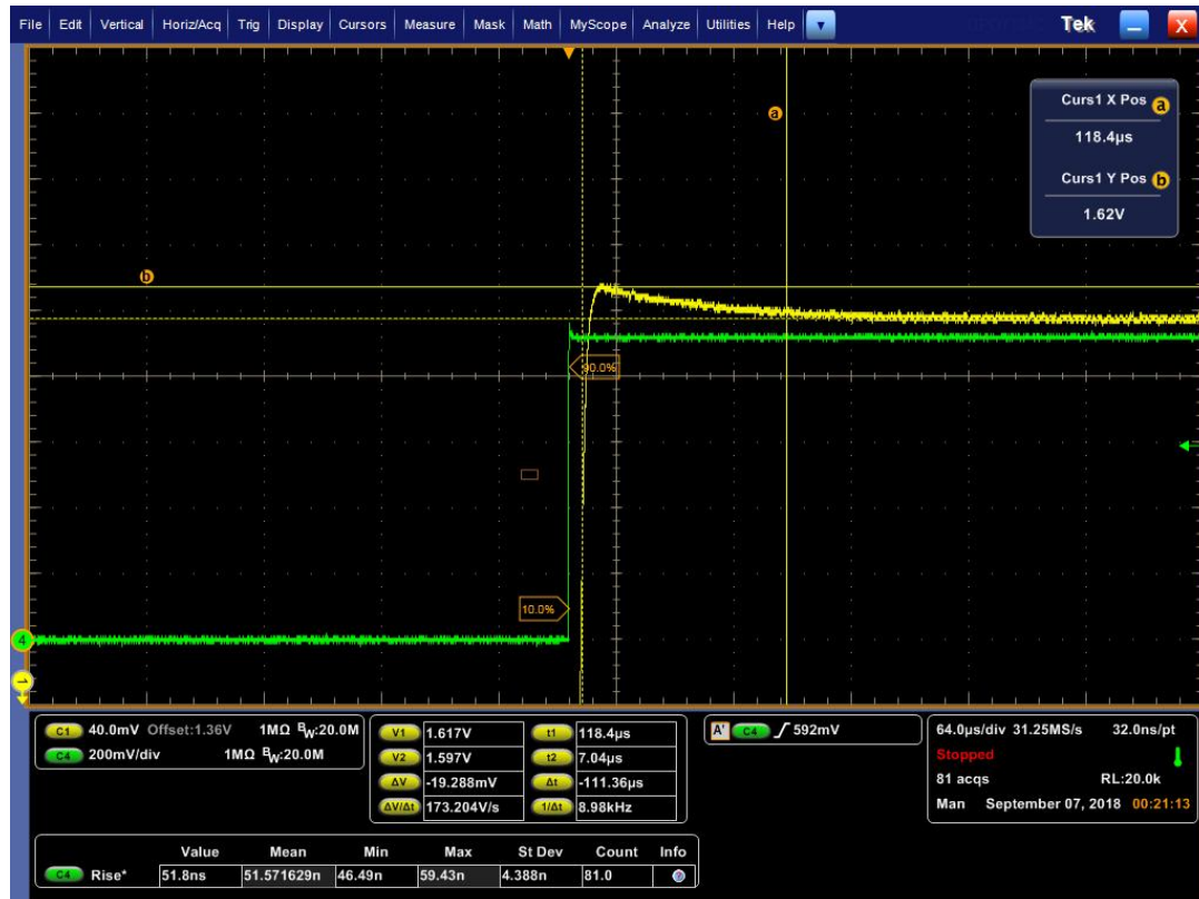
Figure 1-1, 20 channels burst on at same time, -13dBm Per Ch, Monitor one of the channels, Gain excursion:0.5dB
